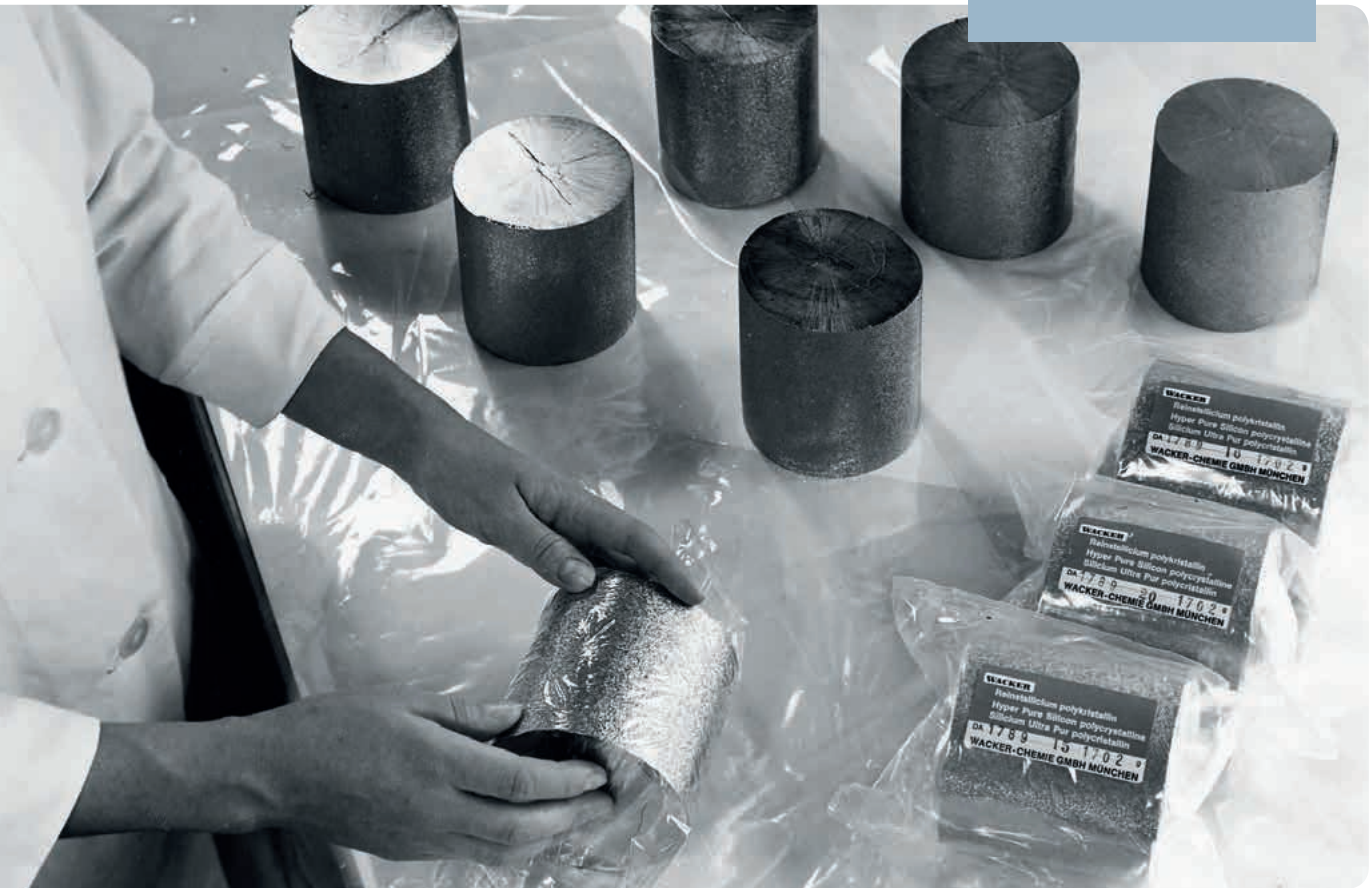
Checking and packing hyperpure silicon in Burghausen, 1965 (above) and dispatch of polysilicon rods, 1968 (below)
