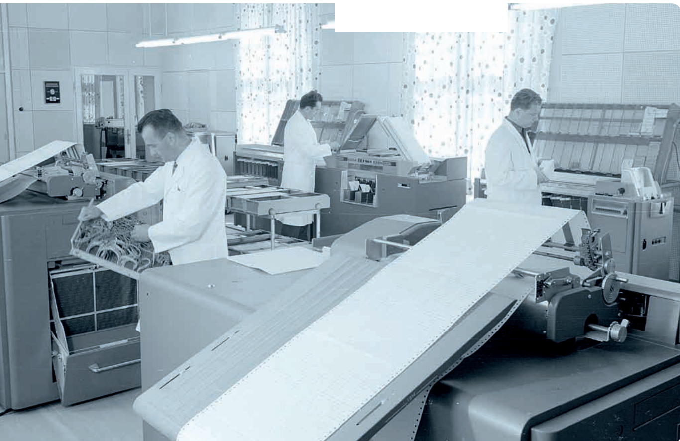
Electromechanical data processing: Hollerith punched card equipment was introduced in Burghausen in 1964. The perforations in the cards were a means of recording and storing data (above), which other machines could then call up and process (below)
