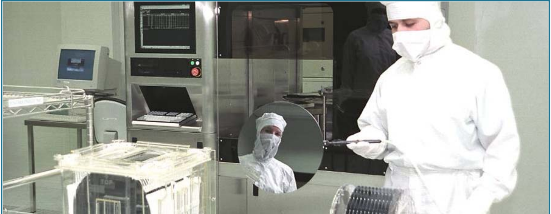
Inspection of 300 millimeter wafers
