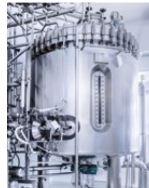
k Proteins intended for therapeutic use from the bioreactor must be purified in several steps. This is done by filtration and chromatography.
