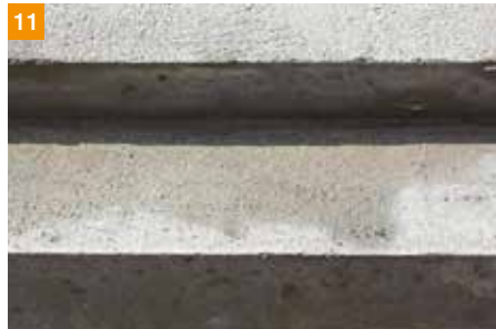
Capillary water uptake of drill cores taken from the Fürstenland bridge in St. Gallen, Switzerland, at varying depths (1-mm thick slices are cut off and inspected). Source: LPM report 17'160-2 of May 28, 1997
