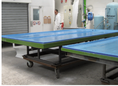
Simultaneous serial production: the molded parts are made on three tables at the same time.
