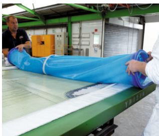
3.1 Removal of bag after curing (2 hours)
