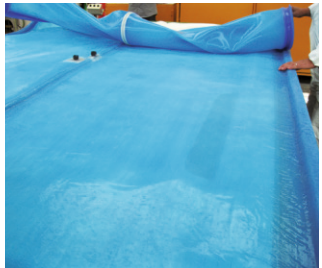
2.2 Covering the fibered mold with reusable vacuum bag
