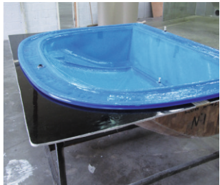
1.4 Spraying the final layer
