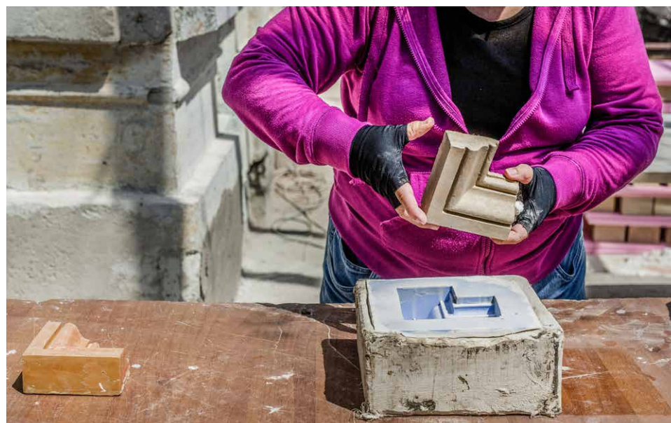
As it is so elastic, the blue silicone mold is placed in a gray support mold made of concrete or gypsum so that a copy can be made.
