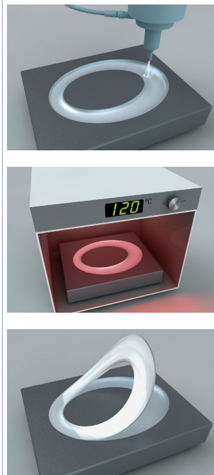
Figure 1: Example of Pelotte Molding Using an ELASTOSIL® P Silicone
