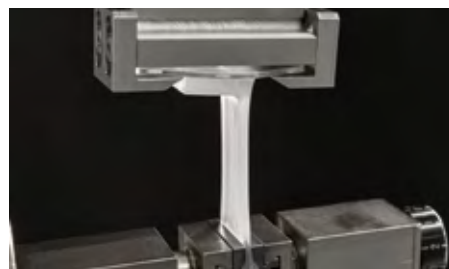
90° Peel Test according to ISO 813
