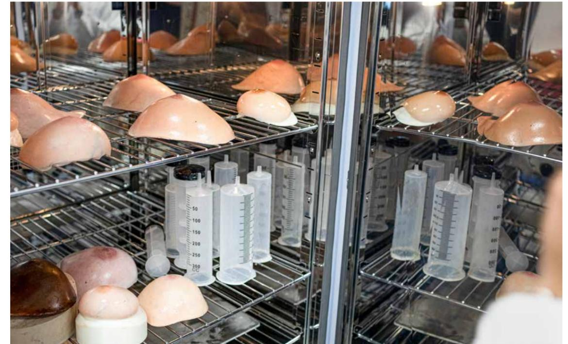
The individual parts of the prosthesis vulcanize in the drying oven.
