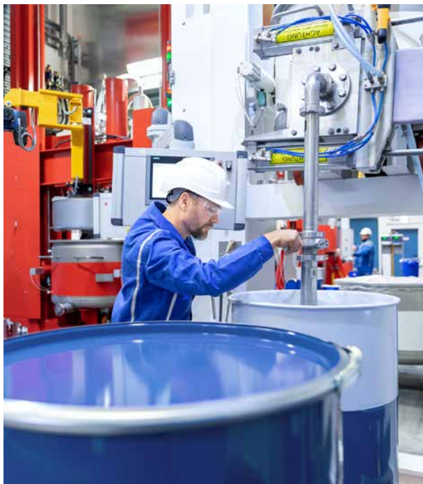
Production of thermally conductive silicone compounds at the Burghausen site. For reasons of quality, the process of filling the transport drums is monitored constantly.
