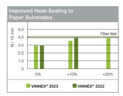
The seal bond strength of PLA and PLA/VINNEX® resin films to paper was determined after heat sealing at 120 °C.
