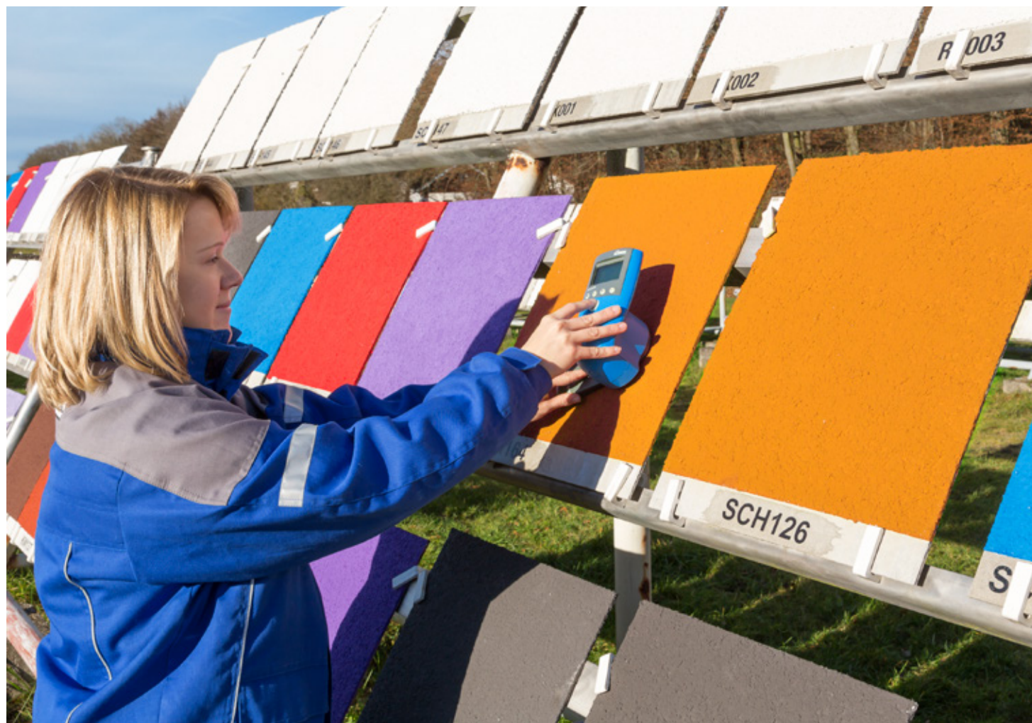
Coated test panels are exposed to the elements for months or even years at the Burghausen plant's open-air weathering facility. WACKER technician Manuela Mühthaler measures at regular intervals how well the various shades of color withstand rain and sun.
