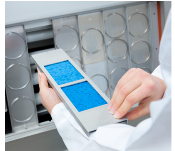
Lab staff use what is known as a QUV tester to simulate accelerated weathering; for this purpose, the test materials are exposed to alternating cycles of UV light and moisture at high and low temperatures.
