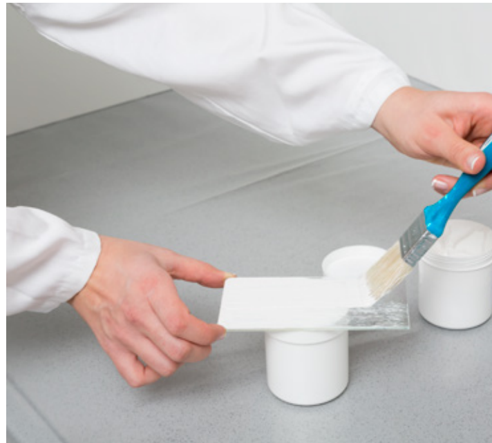
The first step in testing the color fastness of PRIMIS® AF 1000 is to prime test panels in the applications lab in Burghausen.
