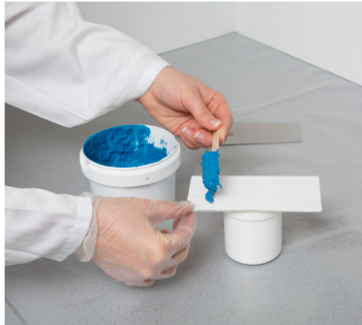
One test panel is then given a coat of paint based on PRIMIS® AF 1000. A second test panel is coated with a commercially available alternative product.
