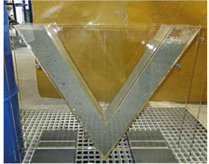
Fig. 1 (left) grit visible in the transparent V shaped mold and Fig 2 (right) illustrates the almost fully filled grit with SFCC, flow direction from the top left wing down and up in the right wing. Inner cross section = 70 mm x 70 mm
