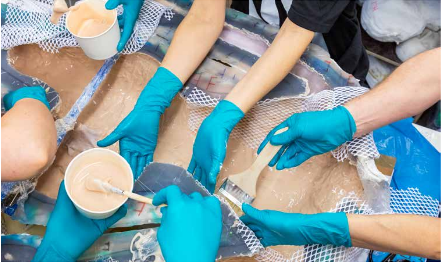
An entire team of makeup artists uses brushes and spatulas to spread the still-liquid silicone over the negative mold.
