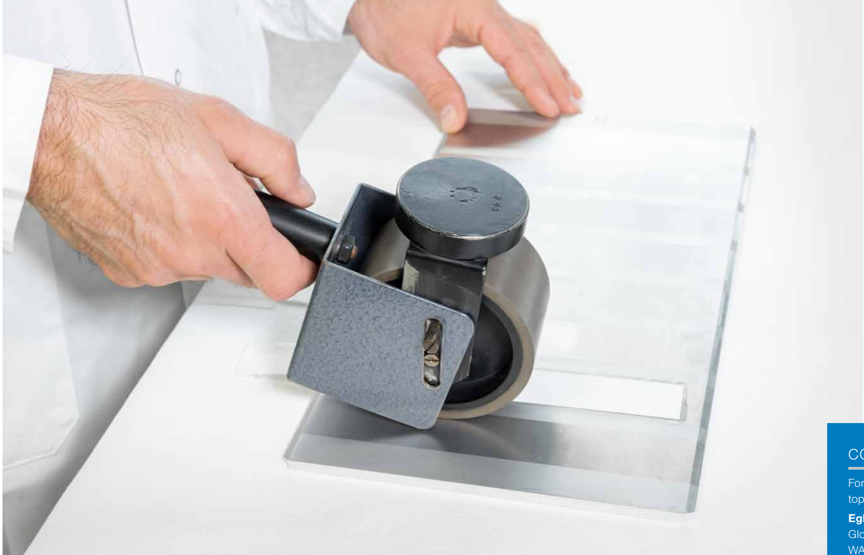
A lab technician using a roller to apply a defined amount of pressure to various test strips in order to determine their release properties.
