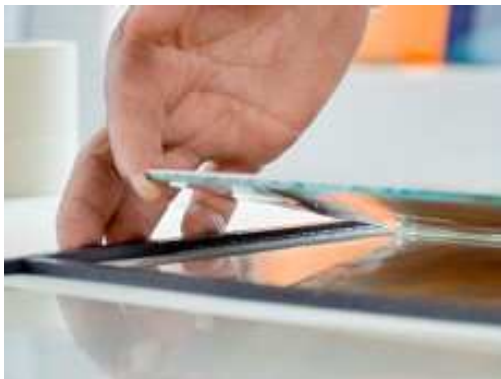
Example: Glass bonding - Carefully laying pieces of colored glass onto the glass substrate.
