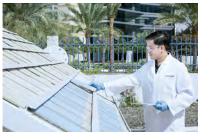
Exterior paints undergoing a weathering test in Dubai
