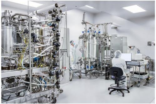
As a CDMO, Wacker Biotech US Inc. operates microbial fermentation lines with a capacity of up to 650 liters for cGMP compliant production and purification of pDNA as well as pharmaceutical proteins (Photo: WACKER).
