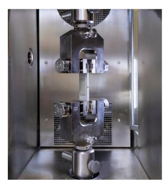
Crack-bridging test according to EN 14891: Waterproofing membranes formulated with VINNAPAS® 754 ED and VINNAPAS® 764 ED can compensate for cracks even at temperatures below freezing, thus reliably protecting the building from water penetration. (Photo:WACKER)
