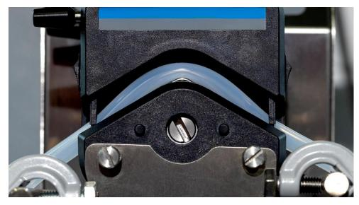
Solid silicone rubber from WACKER can be used, for example, for tubing in heart-lung machines and peristaltic pumps (photo). At COMPAMED, the company will be showcasing products that are particularly suitable for such applications. (Photo: WACKER).
