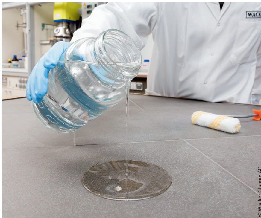
Figure 6: Application of a transparent waterproofing membrane based on Geniosil XT 50.
