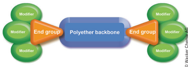
Figure 3: Schematic representation of the end-group modification concept. By selecting different silane modifiers, the properties of the polymer can be varied.
