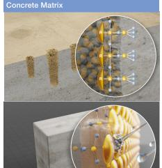
permeability, and long durability, which stems from silanes' high resistance to external influences such as UV radiation, thermal stress, aggressive substances, and microbes. This is due to extremely stable covalent bonds between the silane and the silicate matrix of the pores and capillary walls in the concrete.
