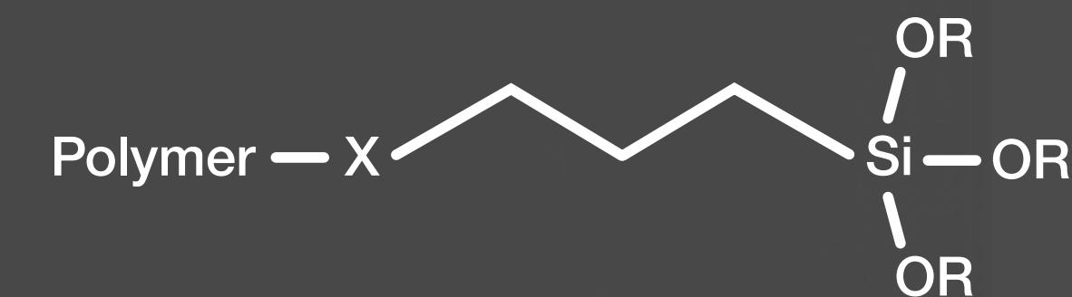
Rather than a propyl group, WACKER organofunctional  $\alpha$ -silanes have a very short methyl or  $\alpha$ -spacer linked to the silicon atom. As a result, the organofunctional groups are much more reactive. And the same applies to the corresponding  $\alpha$ -silane-terminated polymers: they can cure 100 – 1,000 times faster and do not need tin catalysts.
