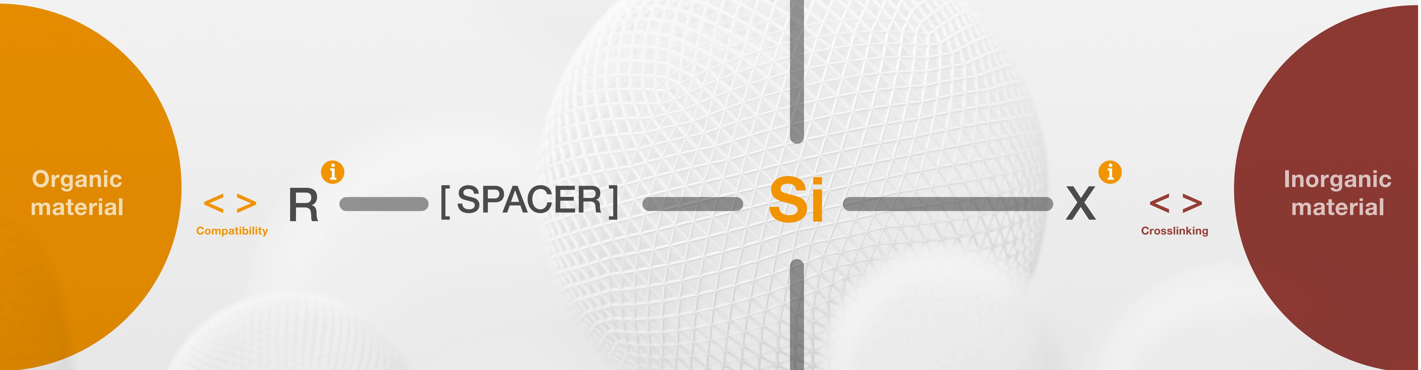
Organofunctional silanes combine the functionality of a reactive organic group with the inorganic functionality of an alkoxy silane in a single molecule. They can act as molecular bridges between organic polymers and inorganic materials (e.g. glass, metal, ceramics).
