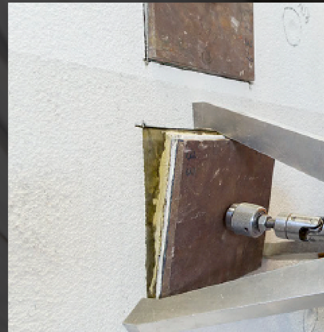
Afterwards, the system is inspected to detect failures such as cracks. Adhesion strength is tested here. Water absorption or impact resistance can also be tested.
