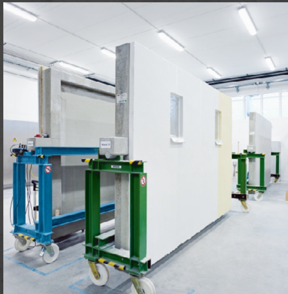
Walls are prepared with a complete ETICS.
