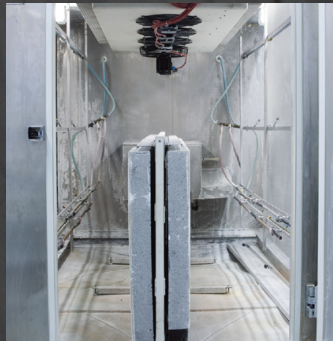
The wall is then subjected to defined hygrothermal cycles for a defined period of time in an EOTA chamber.
