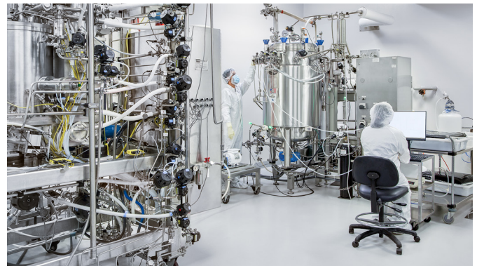
Wacker Biotech's pDNA production site in San Diego is equipped with 43-L single-use bioreactors and 650-L stainless-steel fermentation vessels, including continuous cell lysis.
