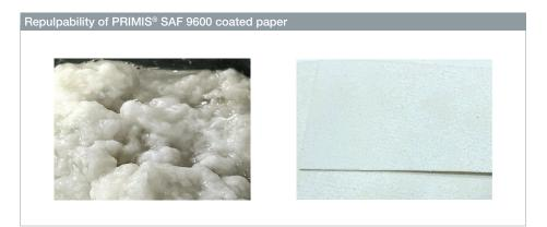
PRIMIS® SAF 9600 does not interfere with paper and paperboard recycling; this enables high rates of fiber recovery and allows consumers to contribute to a circular economy.
