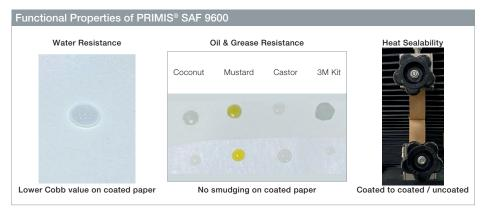
PRIMIS® SAF 9600 exhibits excellent heat sealability, good water resistance and oil & grease resistance upon suitable formulation.
