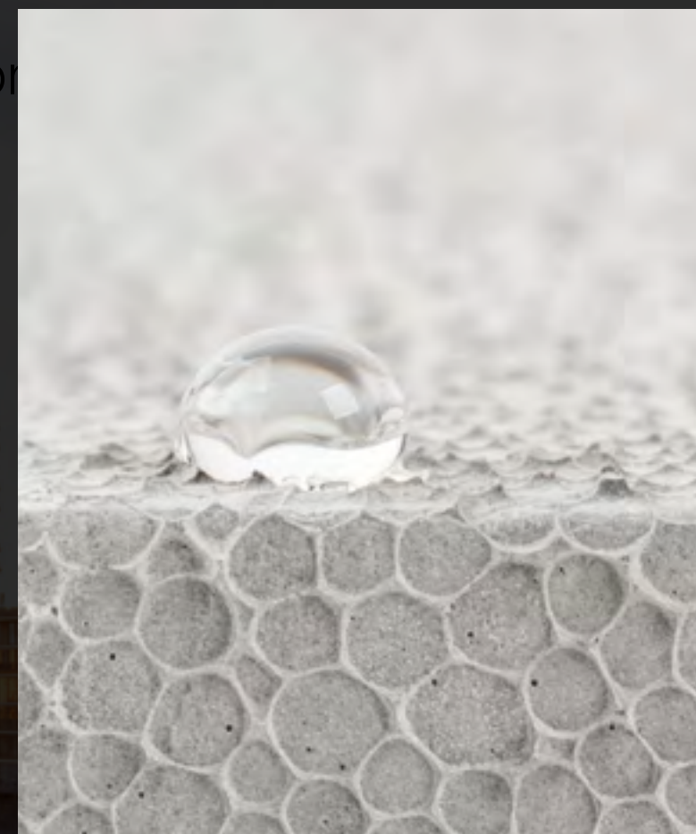
When a hydrophobic impregnation is applied, the water beads off.
