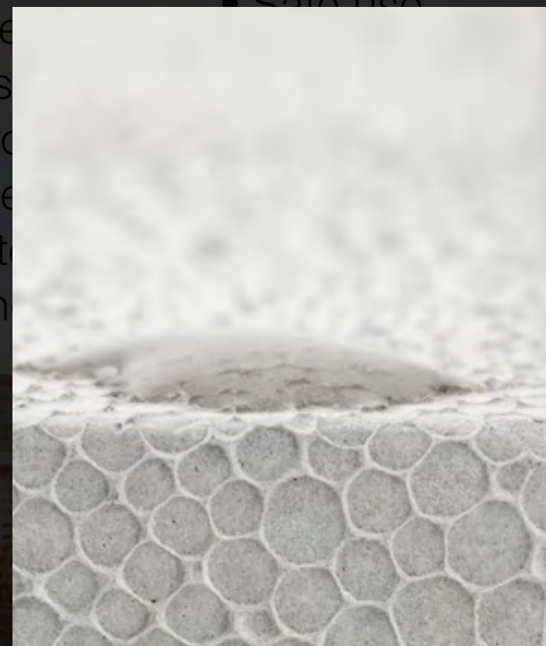
The untreated substrate absorbs water.
