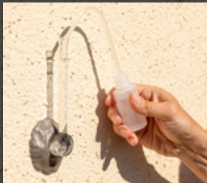
The Karsten tube test simulates a downpour in strong winds. The water does not even penetrate via cracks in the walls.
